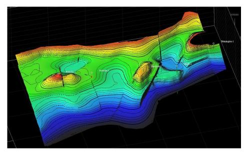
Map of the Silkstone Coal (Westphalian) illustrating the location of five of the wells drilled in Derbyshire. The Hardstoft discovery well is located on the anticline in the centre of the image
