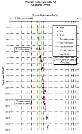
Figure 1. Vitrinite Reflectance measurements performed on drill cuttings from the Salsburgh- 2 well. When the data is extrapolated to surface the shale has an Ro of close to O.6 indicating approximately 6000 ft of inversion.
